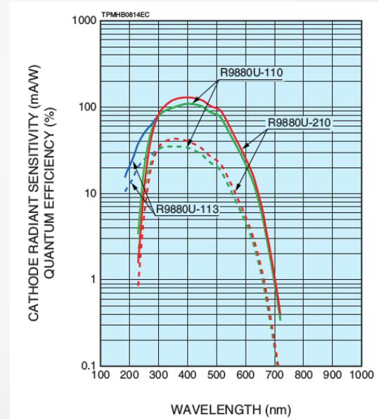
High Gain, fast time response and high quantum efficiency
