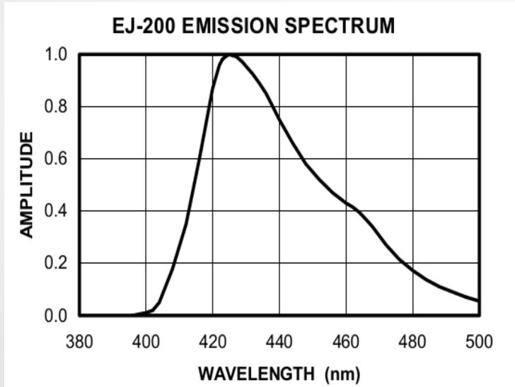
EJ-200 plastic scintillators combines a long attenuation length, a fast timing and high light output
