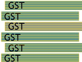
**Structure** → tendency of Sb<sub>2</sub>Te<sub>3</sub> in SL grown by MBE to incorporate GeTe
