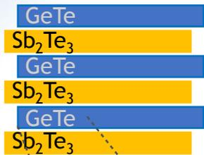
Structure → SuperLattice (SL) – alternation of (GeTe)<sub>2</sub> and Sb<sub>2</sub>Te<sub>3</sub> blocks
