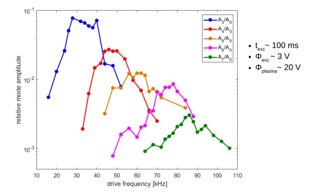
In this work, we show an experimental technique to control Kelvin-Helmholtz modes of arbitrary wavenumber by rotating electric fields in magnetized nonneutral plasmas. The results are in good agreement with theoretical predictions, proving this technique to be a useful tool in the study and control of fluid instabilities. In the future we are going to
