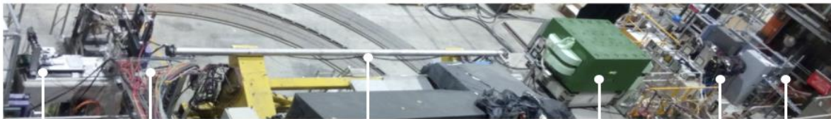
target Be or C Si microstrip stations vacuum beam pipe dipole magnet CAL DT
