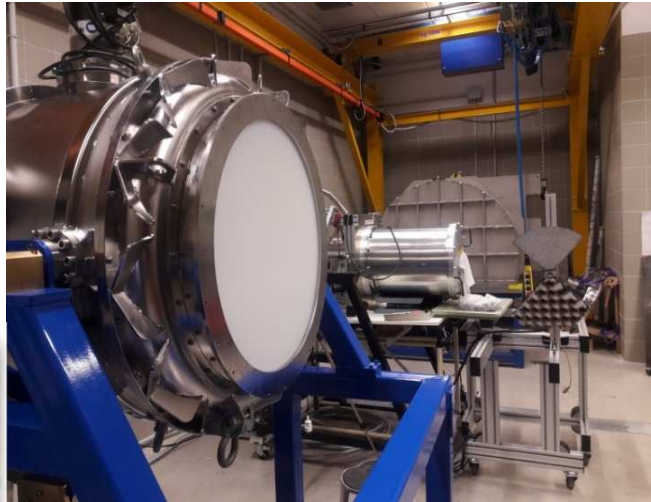
Cryostat and vacuum window
