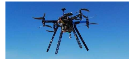
Drone-based beam calibration (CNR/TO)
