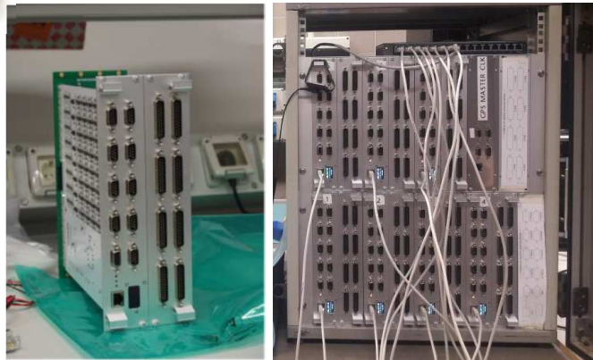
Electronics (BIAS board and DAQ)
