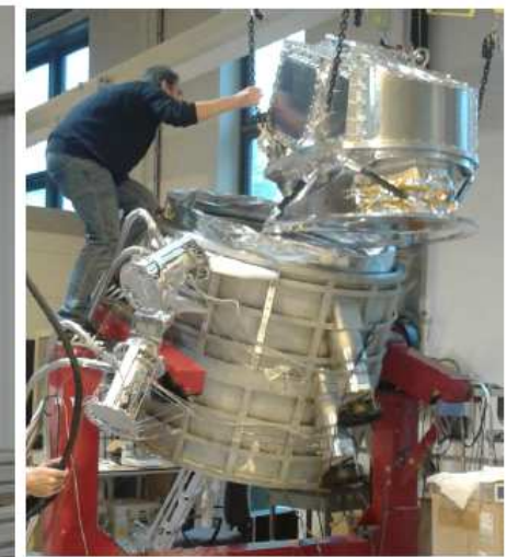
Integration of the 1K box in cryostat shell
