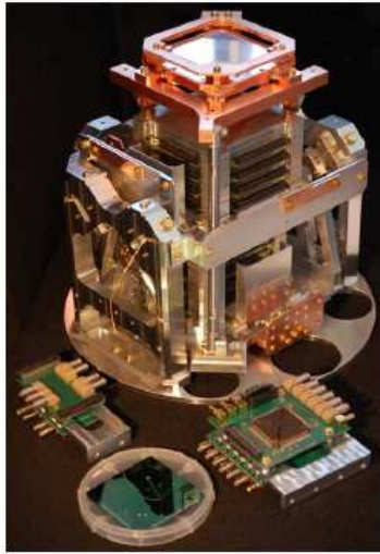
Cryogenic section of the detection chain
