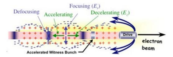
In this scheme a driver beam creates a plasma wake, while a witness bunch is accelerated in the back of the plasma bubble. The aim of the experiment is:
