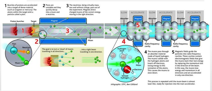
A cooling cell consists of a sequence of LiH or liquid hydrogen absorbers within a lattice of up to 3.5 T solenoids that provide the required particle focusing
