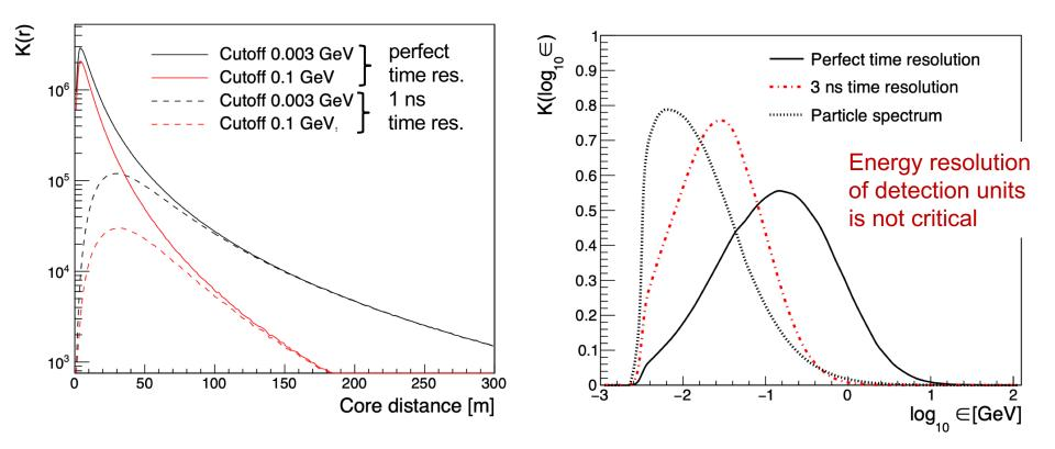
Time resolution of some 10 ps Position resolution of some cm Detection efficiency for gammas >50% above ~100 MeV Minimal or no energy resolution CAN SUCH A DETECTOR BE BUILT?
