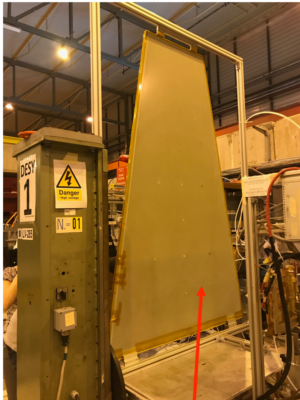
GE2/1 20 o sector with M4 \mu RWELLs (2m height, 1.2 m base)
