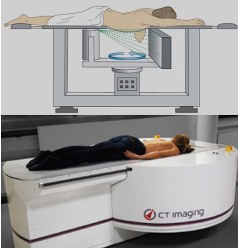
A breast CT scanner with the patient in prone position with one breast being imaged at a time (typically 10 seconds or less) and without compression. Image courtesy of Dr. Willi Kalender
