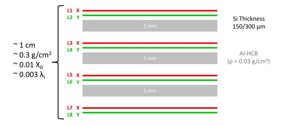
The geometry is fully parameterized (thicknesses, gaps, ...), i.e. decided in production. This layout is not realistic, but it is still **good for basic estimations** of resolution.
