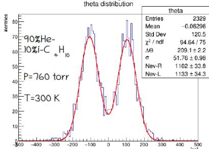
$$\Delta\Theta = (209.1 \pm 2.2) \text{ ns} \quad v_d = (1.91 \pm 0.02) \text{ cm}/\mu\text{s}$$
