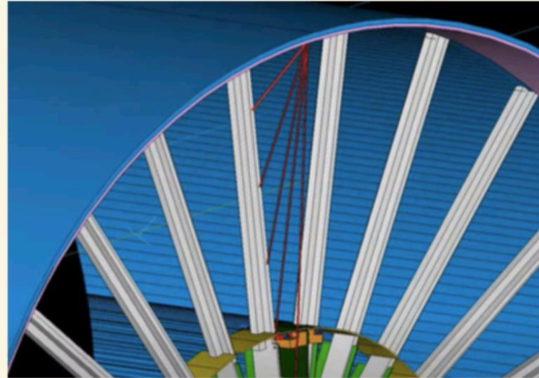
To fix the tie rods at the inner cylinder we will use a pin
