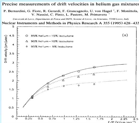
For a 90/10 mixture, at normal pressure, variations of the electric field, around the operating value of 1 V/cm/torr, of about 2 V/cm induce drift velocity variations of  $1 \times 10^{-3}$ .
