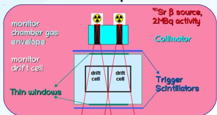
The chamber can be supplied with gas coming from the inlet and the outlet of the detector.
