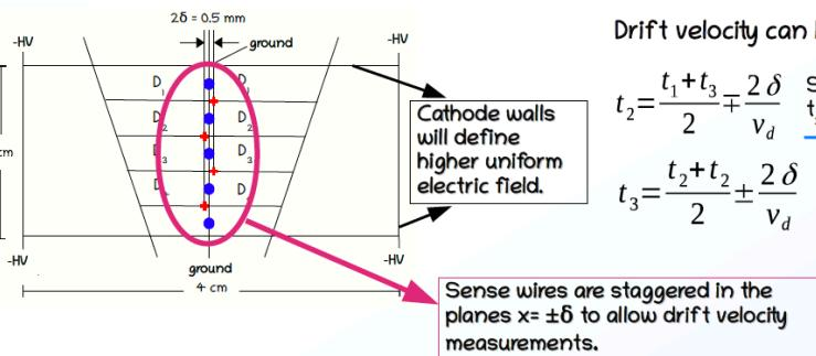
Drift velocity can be measured using the shift on wire positions, starting by time relations:
