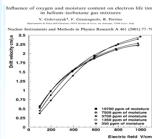
To mitigate the ageing effect, sometimes it is useful to introduce small quantities of water vapors in the gas mixtures, but it is important to control the consequent variations of drift velocity.
