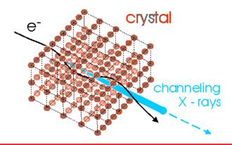
The **Baier-Katkov** method permits to simulate the emitted radiation in crystals in a wide energy range, from **sub-GeV** to **hundreds** of **GeV**.
