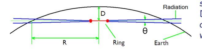
Radiation from ring exits on a phisymmetric corona. (Plot: M. Palmer) Due to Earth curvature, linear dimensions along the local "meridian" are stretched with respect to perpendicular
