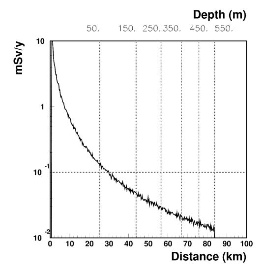
FLUKA results for ambient dose equivalent  $(H^*(10))$  as a function of distance from ring, or (top axis), depth of the ring. Averaged over 1m in the vertical plane. Assuming 1.2 10  $^{21}$  decays/y (2.10 $^{12}$   $\mu$ /bunch, 15 Hz, 200 days)
