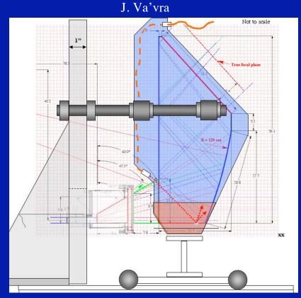
• Fiber comes to a bulkhead fiber connector in easily accessible spot, and the continues as another segment ending in the lens, producing parallel pencil-like beam. The beam is reflected from a small piece of etched aluminum glued to the bottom of FBLOCK.
