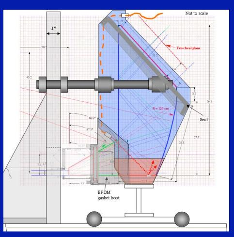
• Need to flow N<sub>2</sub> gas around the FBLOCK's surfaces to prevent the a moisture condensation and the pollution accumulation on the surfaces.
