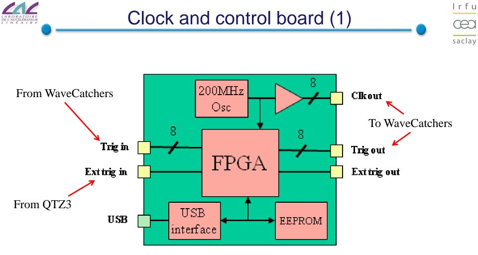
CRT mode : when the controller board detects a coincidence between an external trigger from QTZ3 and one of the sixteen channels, it sends through USB a specific interrupt to the PC in order to start the data readout.
