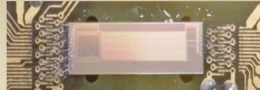
FE chip first results 32x128, 50 um pitch
