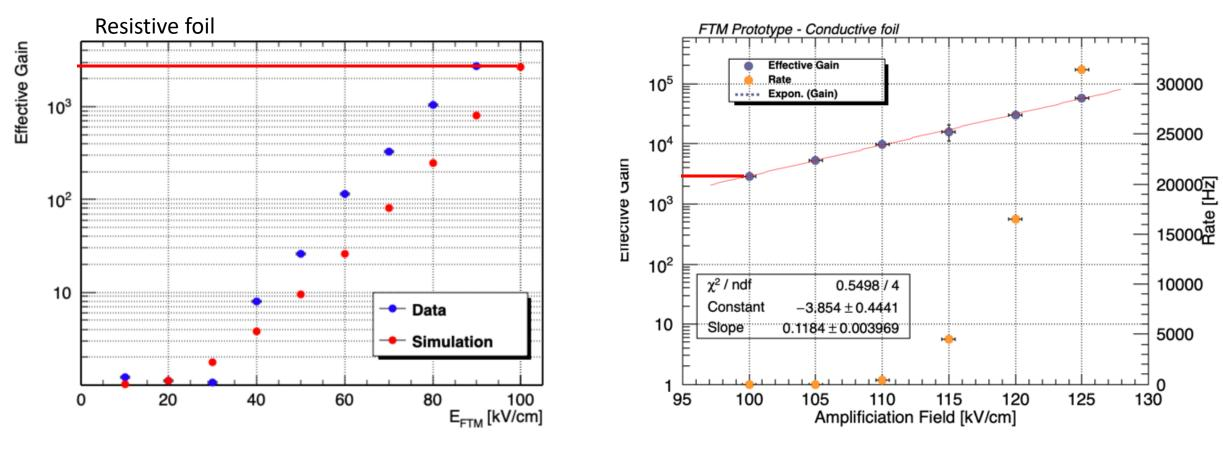
If indeed the #primaries is around 346 (to be confirmed) then we are in a good agreement to what have been measured Also for the resistive foil and the simulation
