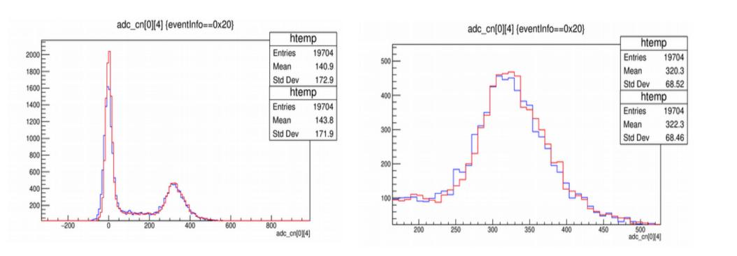
The MIP signal is located around 320 ADC, so the expected S/N ratio is about 21
