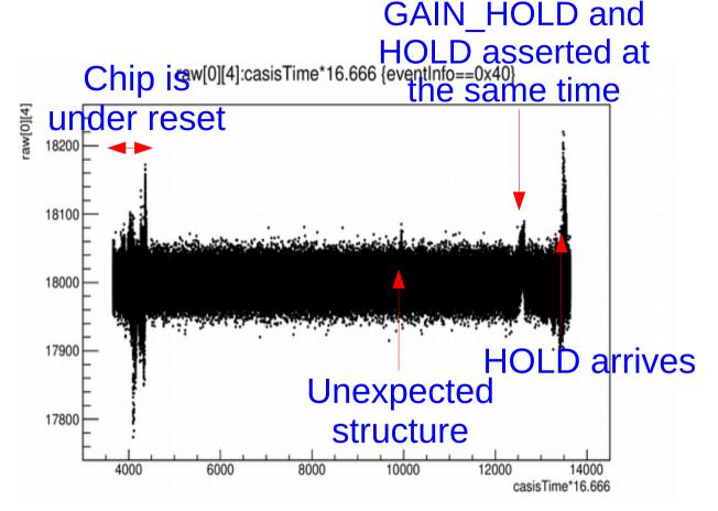
According to suggestions from Trieste colleagues, the simultaneous signals GAIN\_HOLD and HOLD could interfere with the analog signal at the board or chip level: what we can do for the moment is to not assert GAIN\_HOLD signal when it would arrive synchronous or delayed respect to the HOLD signal.
