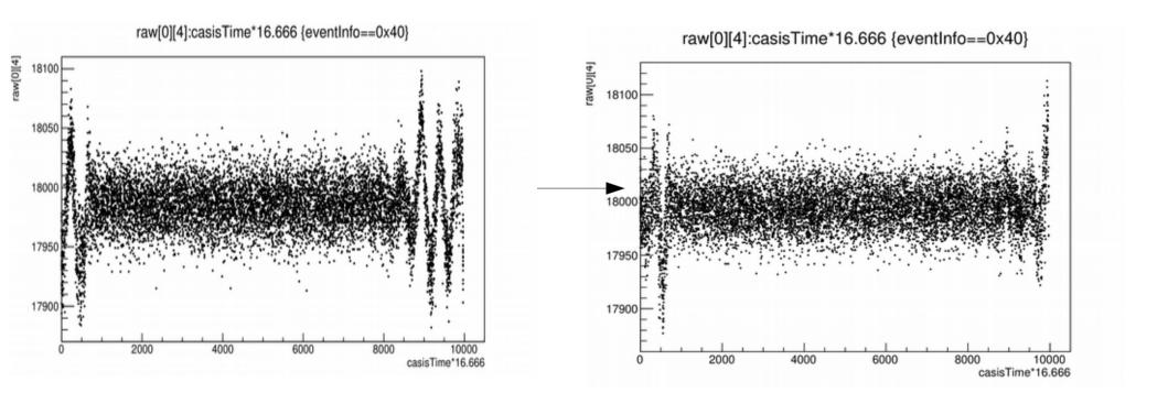
Batteries work much better than Keithley in reducing the external interferences, but they are not very comfortable...
