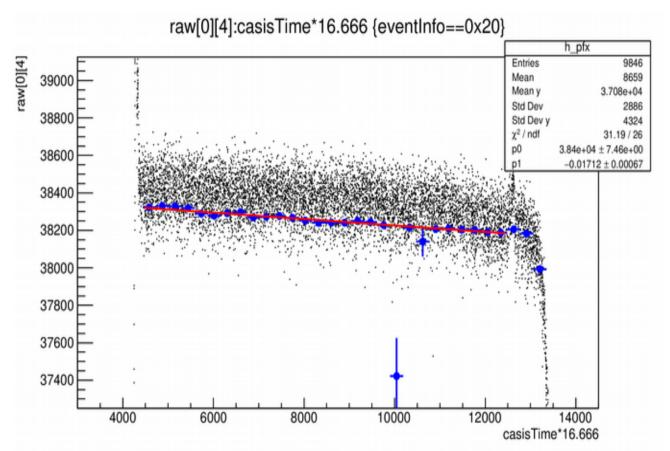
The signal decrease as a function of CASIS Time means that, enlarging the integration window, the integrated signal increases by 0.0171 ADC/ns.
