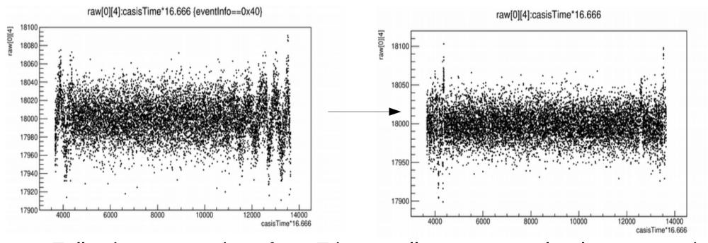
Following suggestions from Trieste colleagues, we clearly separated digital signals from analog signals on the experimental table. Additionally, we used a power supply filter made by Sebastiano that gave us a result only slightly worse to the batteries one.
