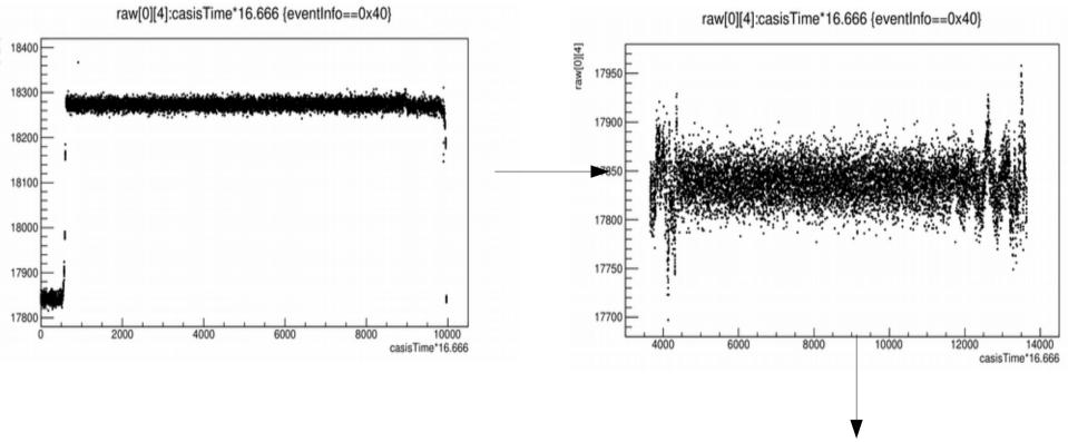
The casisTime has now an offset of 220 clock counts, problem that was solved in version V2514 (but all data shown here was obtained using previous firmware)
