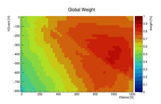
The voltage values of sense and guard wires for a uniform electric field inside the drift cells are:
