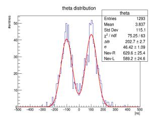
The drift value extrapolated from this distribution is:  $v_d = 1.97 \pm 0.03 \text{ cm}/\mu\text{s}$
