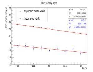
There is still a shift between theoretical value and experimental value of drift velocity.
