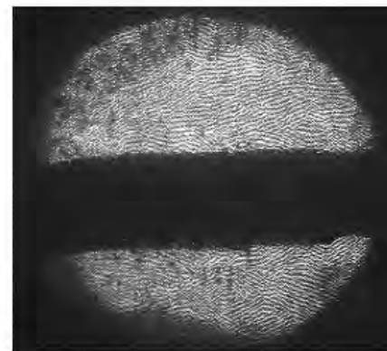
Hg-jet - beam impact 4 \times 10^{12} protons, 10T field
