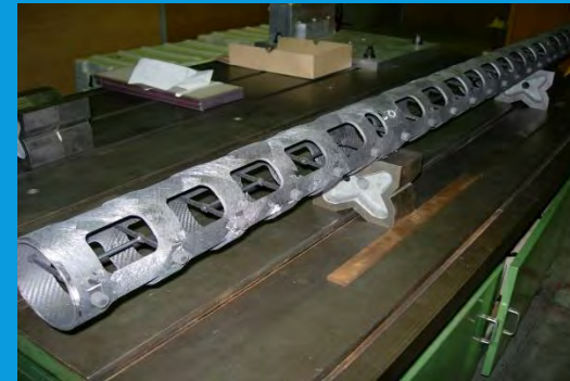
CNGS graphite target assembly (2005, D.Grenier et al.)
