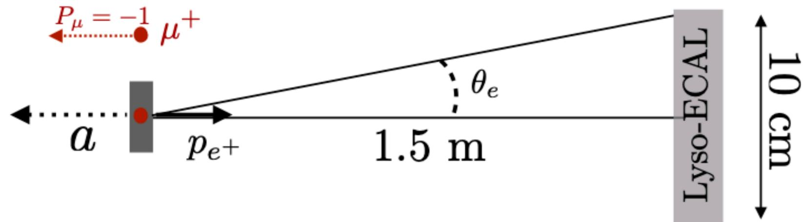
**Figure 5.** The proposed MEGII-fwd set-up. A Lyso-ECAL detector of 10 cm in diameter is placed along the muon beam line 1.5 m downstream from the stopping point. The muon polarization  $P_\mu$  is in the opposite direction than the detected positron.
