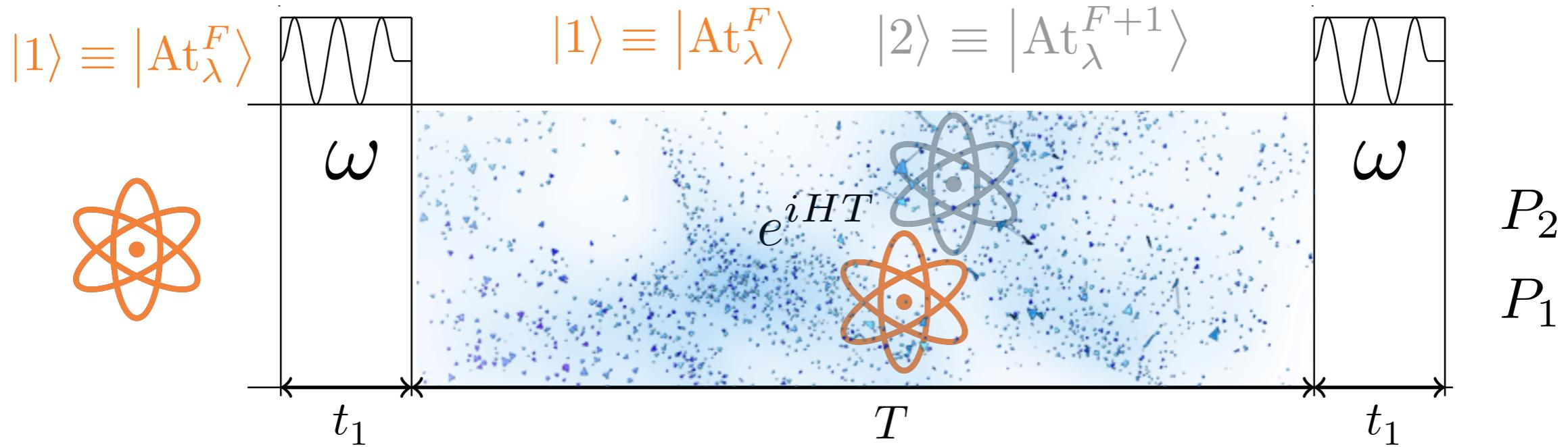
after ‘adjusting the device’:  $P_2 = \cos[\Delta\omega T/2]^2$
