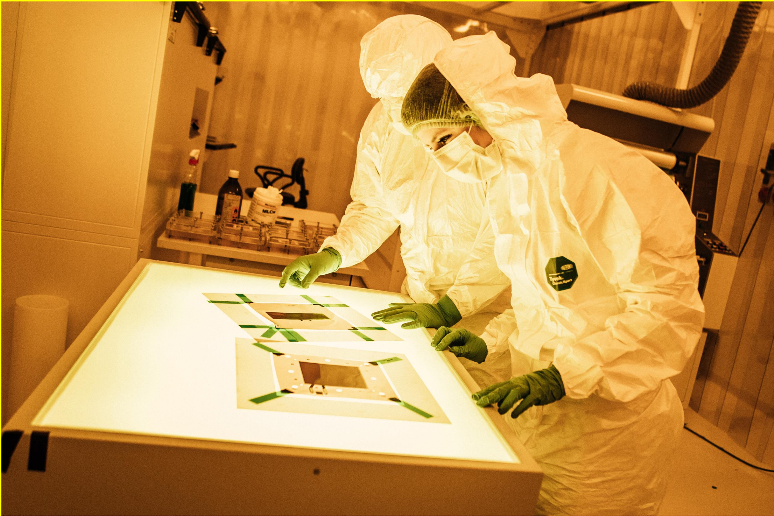
Production of GEM foils according to CERN technology
