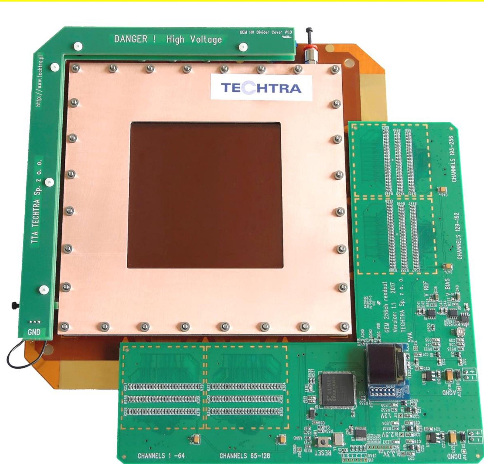
10 x 10 cm GEM detector with 256 ch V1.1 electronic readout
