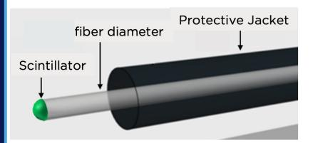
16 optical fiber-based system with scintillating materials on the tip: **Gadox** for LDR and YVO for HDR.
