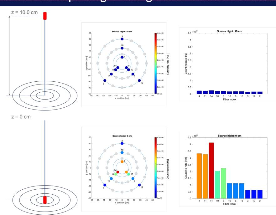
position The Source was reconstructed using triangulation algorithm based on the counting rate measured by every source.
