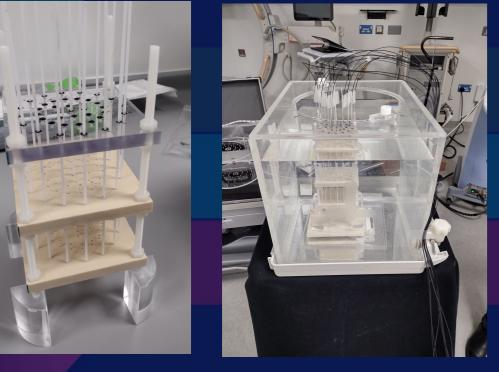
The initial evaluation of the 16-channel system, with sensors placed around a <sup>192</sup>lr radioactive source was performed at the Queen's University Hospital (Belfast, Ireland), using a phantom with a circular geometry in a water tank.
