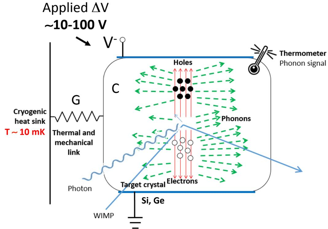
Charges drifting in the electric field produce heating
