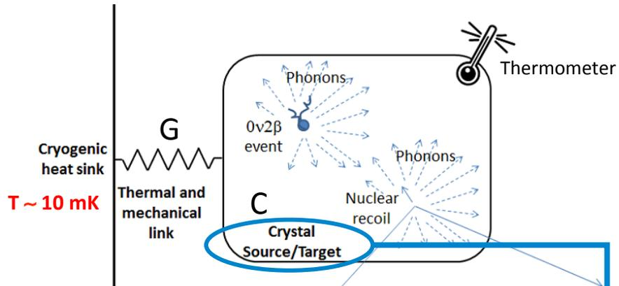
The **energy** deposited by an event into an energy absorber weakly connected to a heat sink determines an **increase** of its **temperature**
