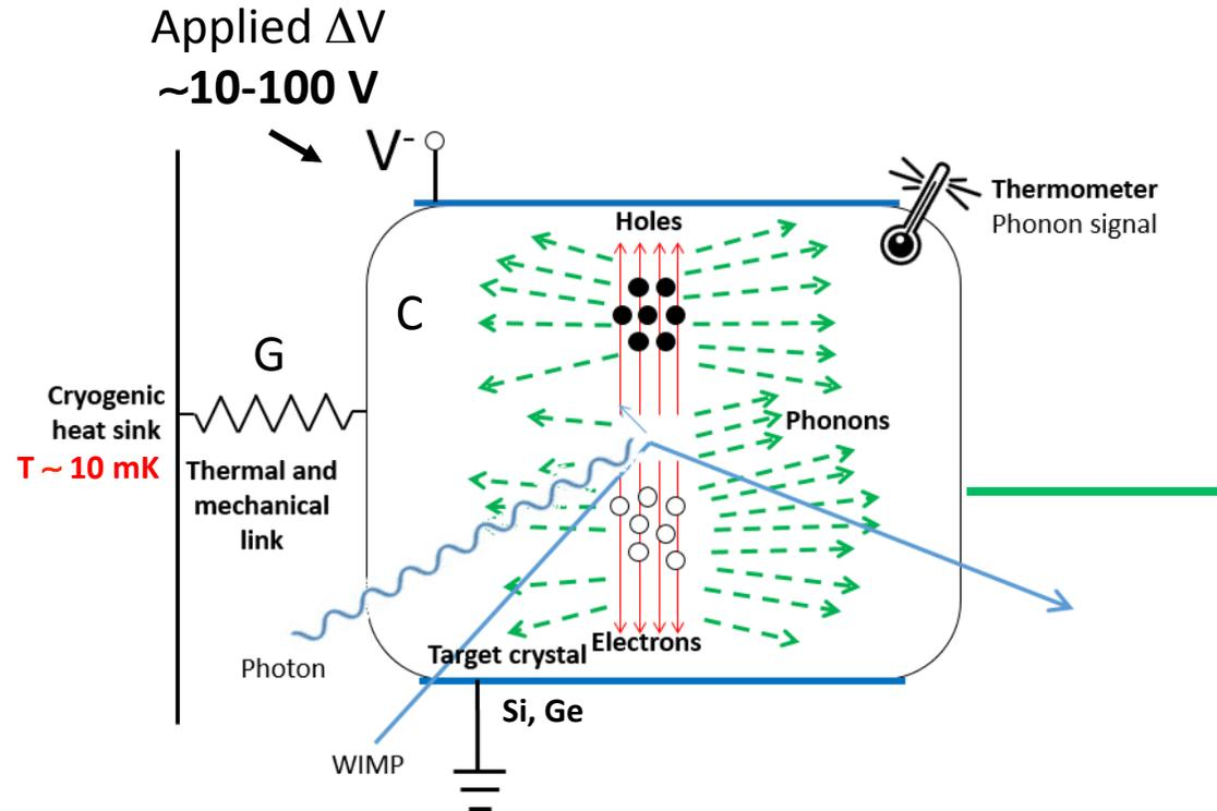
Charges drifting in the electric field produce heating
