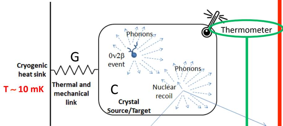
The **energy** deposited by an event into an energy absorber weakly connected to a heat sink determines an **increase** of its **temperature**
