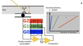
It combines a charge-integrating architecture and three dynamically switching, linear gains per pixel
