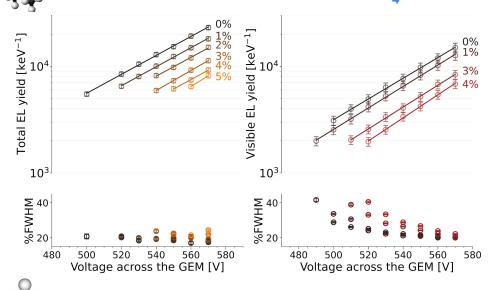
Small percentages of isobutane and methane quench the visible and UV photons emitted by He-40%CF<sub>4</sub>, but they do not completely compromise the optical readout.
