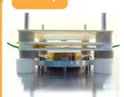
A Large Area Avalanche Photodiode (LAAPD) was used to readout the EL produced in the avalanches of a Gas Electron Multiplier (GEM).
