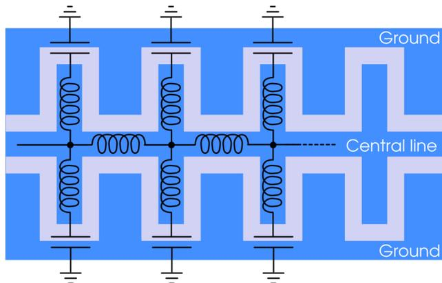
Exploit the non-linear kinetic inductance of TiN or NbTiN
