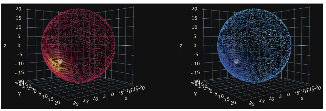
Example of an event seen by 20" PMTs for a positron of 6.165 MeV deposited energy. The color represents the accumulated charge in PMTs (left) and PMT activation time (right). The gray sphere: the primary vertex.
