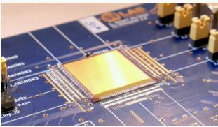
TJ-Monopix2: Proof-of-principle prototype of Belle II VTX
