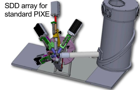
Drawing of the new external beam set-up for atmospheric aerosol analysis at INFN-LABEC, integrating a SDD array with the HR PIXE spectrometer
