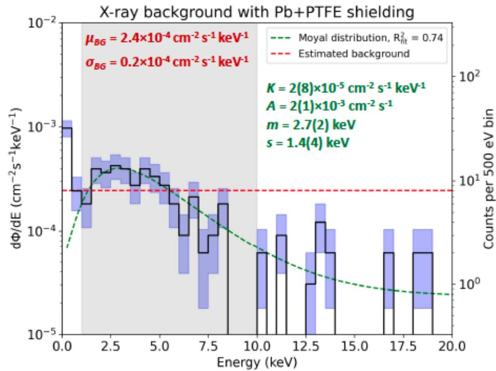
Background measurement with SRON FDM TES array
