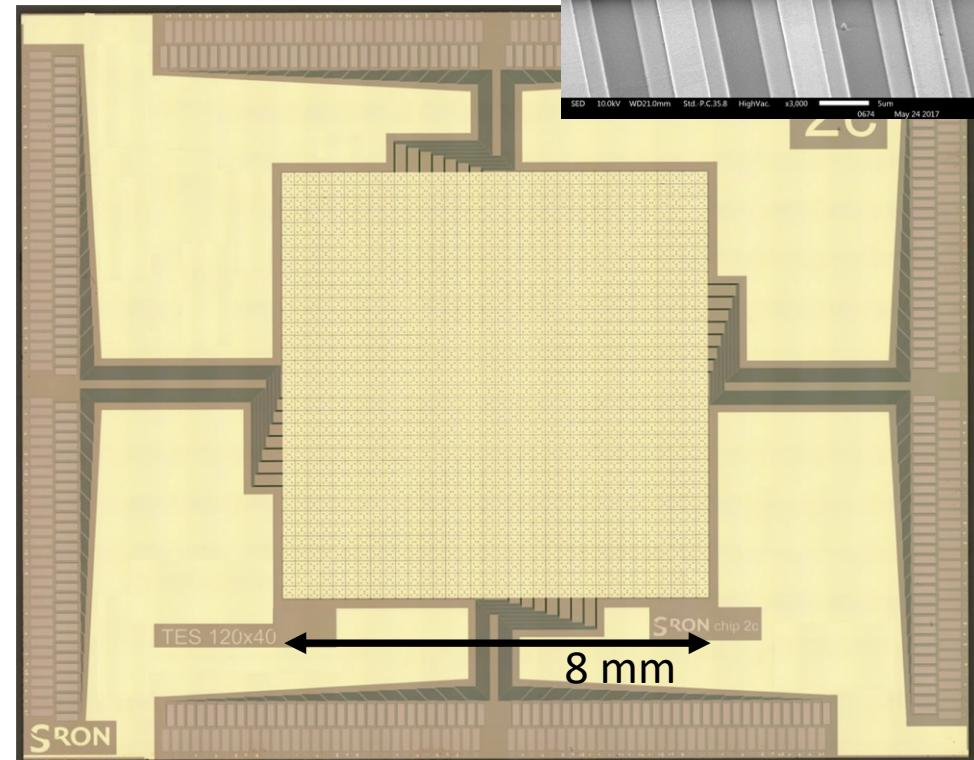
Micrograph SRON 32x32 array before absorber deposition
