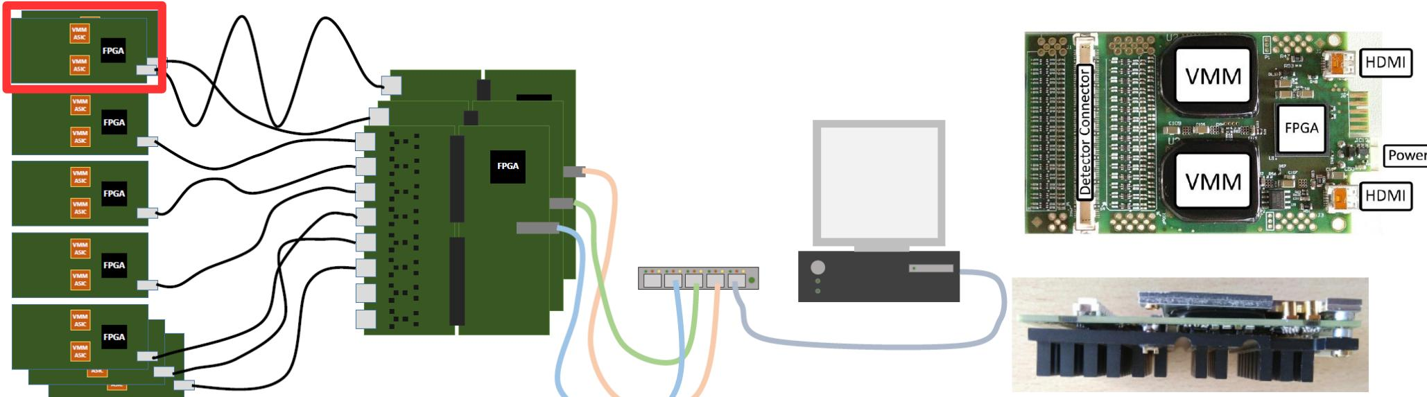
VMM Hybrid → HDMI cable → Adapter card + FEC → Ethernet → Switch → Ethernet → PC
