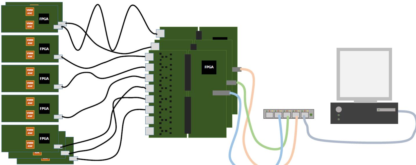
VMM Hybrid → HDMI cable → Adapter card + FEC → Ethernet → Switch → Ethernet → PC
