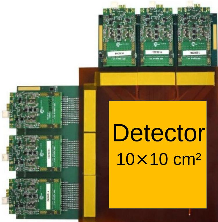
First test layer front-end electronics.
