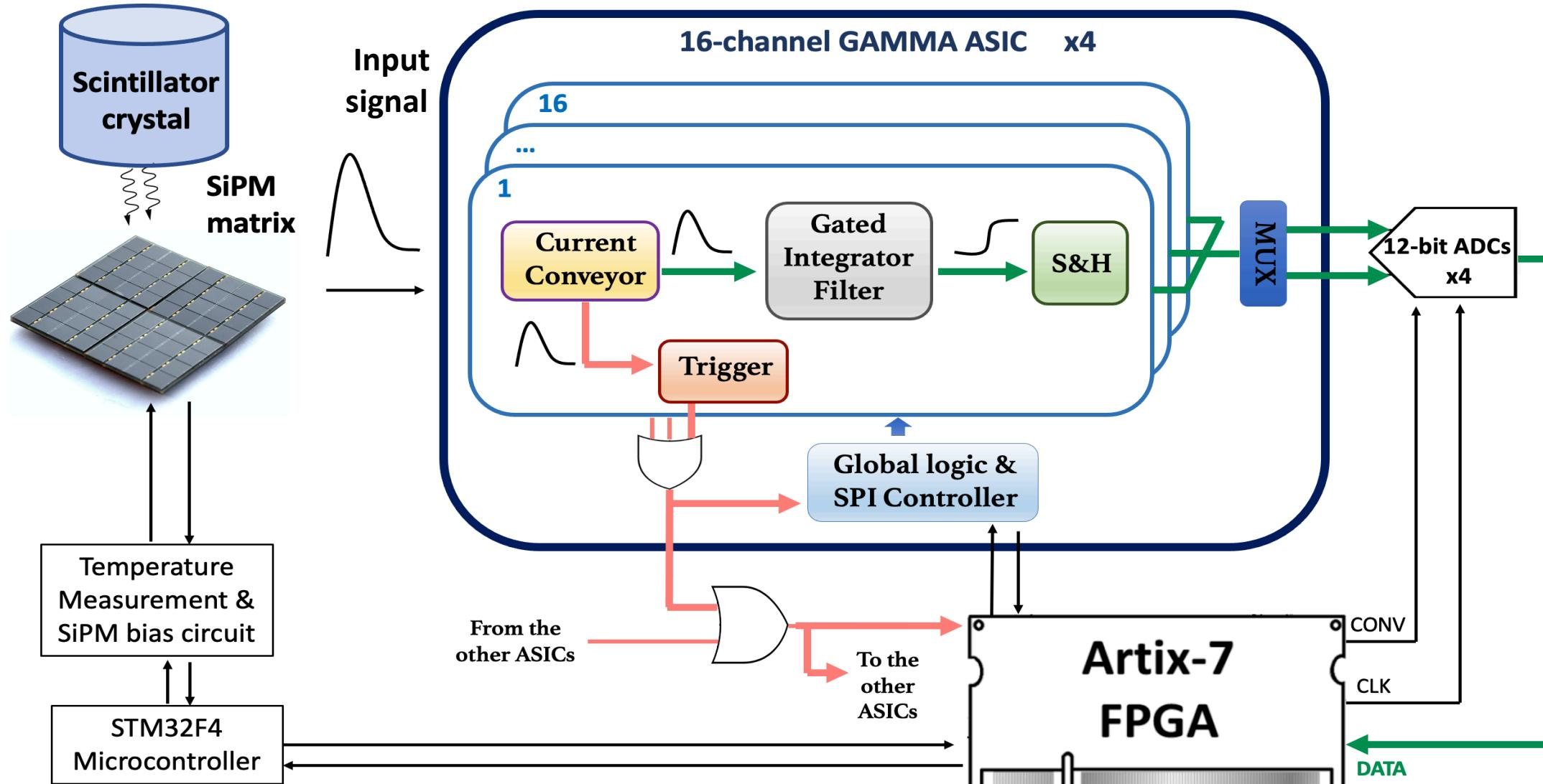
1. Compatible with large SiPMs ( $\sim$ tens fF); 2. Gain modulation allows for **84dB** Dynamic Range on each channel
