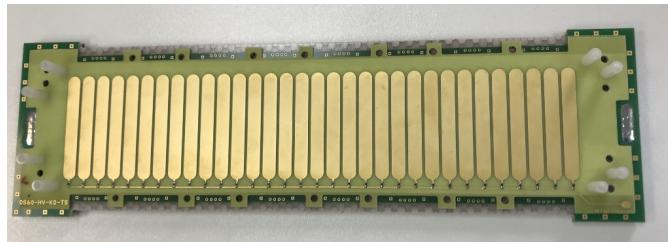
Anode readout electrode
