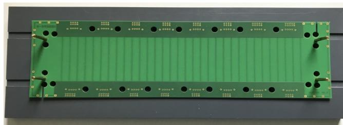
Cathode readout electrode
