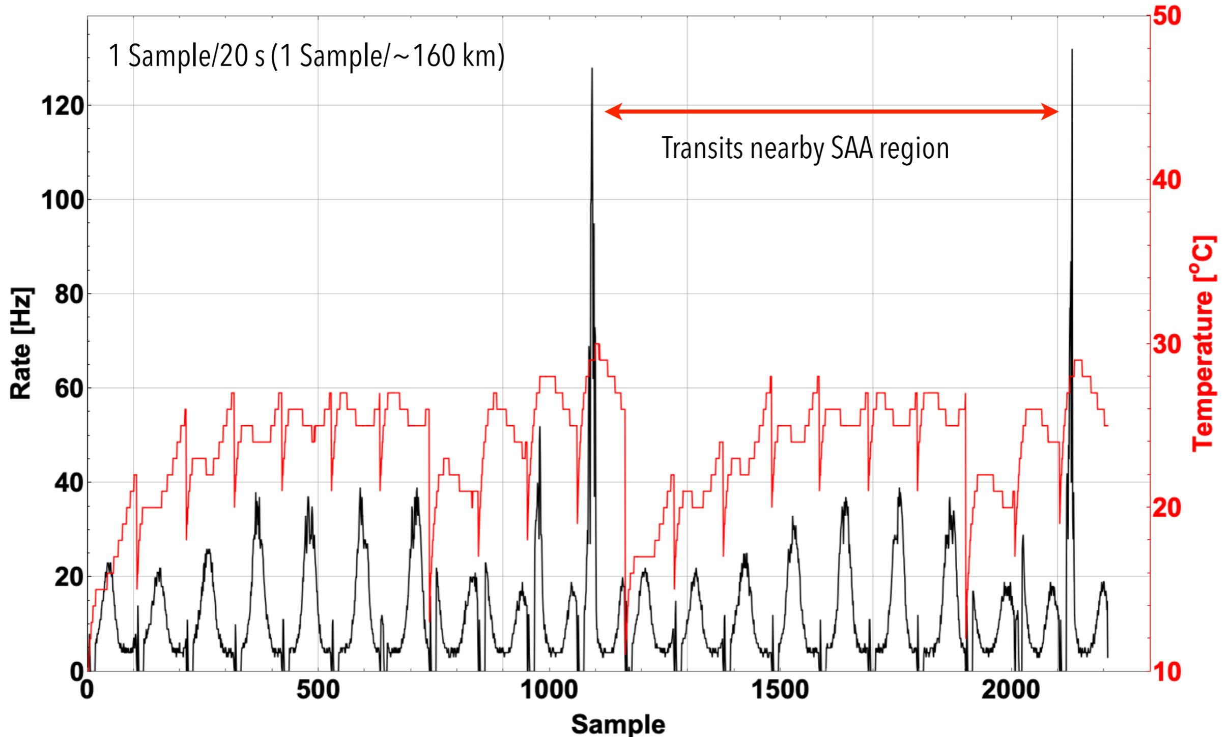
SiPM CH2 detection THR set to 1800 ADC CH / 64k ADC CH
