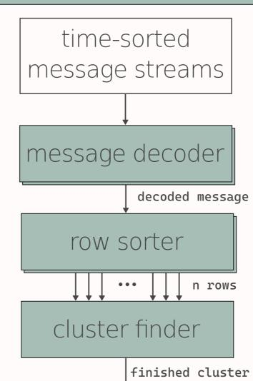
message frames are decoded in the message decoder, where the message frames are combined into a single trigger message. In the decoding step, the data undergoes a baseline correction, the maximum ADC value is extracted, and a more precise reconstructed. signal time is Additionally, pile-up is detected and removed from the message stream for a potential pile-up reconstruction.
