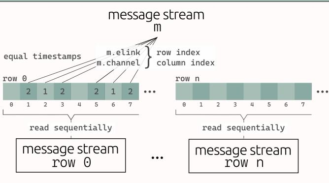
The next step is to **sort the data** stream according to the pad configuration, this Will as significantly simplify the cluster
