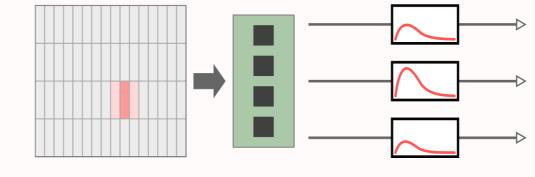
Schematic depiction of a detector trigger, where the center pad fulfilled the SPADIC trigger logic and the neighboring pads are read out as forced neighbor triggers.
