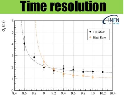
O(1 ns) time resolution obtained with different sRPC prototypes
