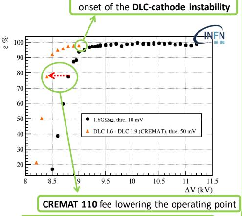
Exploited as a lock-pick for the study of the DLC as SRPC electrodes
