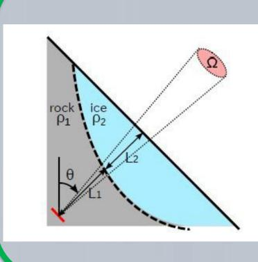
Measuring muon fluxes with good angular resolution allow for glacierbedrock interface depth.
