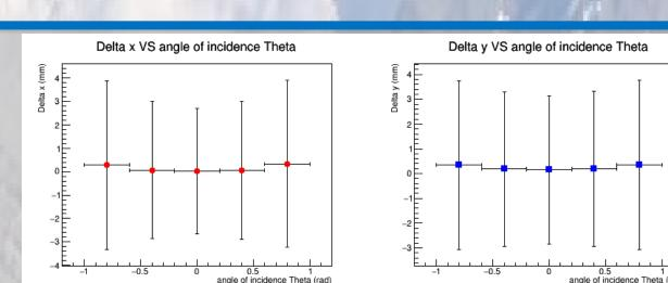
Simulation results show an angular resolution for muon directions of 5mrad on both polar and azimuthal angle.
