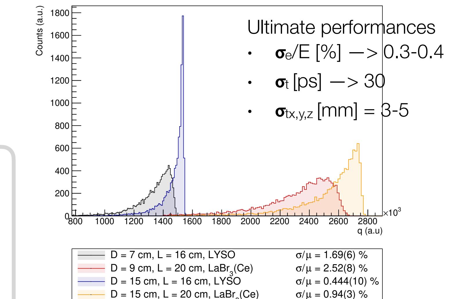
Photons detected per SiPM on the inner surface of an ultimate big crystal
