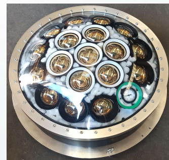
12 mm-thick vessel resisted to 1.3 MPa (Constrain: 1.26 MPa)
