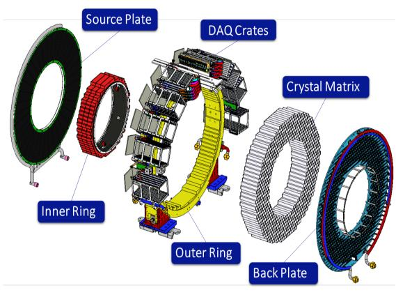
Exploded CAD view of one Mu2e EC disk
