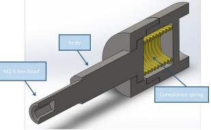
3) Screwdriver: It allows to unscrew the 4 screws. The screws will be locked inside the FE Unit, because of design and the amount of torque (0.083 Nm) is set by the motor current. An axial spring assures compliance during the approach movement, while the transversal positioning is made easier with a countersunk hollow on the screwdriver tip
