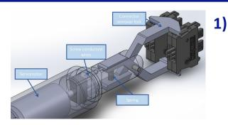
**Connector remover:** It dismounts the two connectors at the same time, pushing the two lateral clips that tighten the connector to the FE board. It has a spring mechanism to ensure grip also in case of lack of power supply and to calibrate di amount of pressure used. A screw-nut mechanism control the plies displacement.
