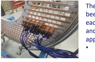
The optimal routing technique found has been to distribute cables horizontally, and each bundle supply the adjacent upper and lower rows of FE Units. It will also apply for the optical fibers.
