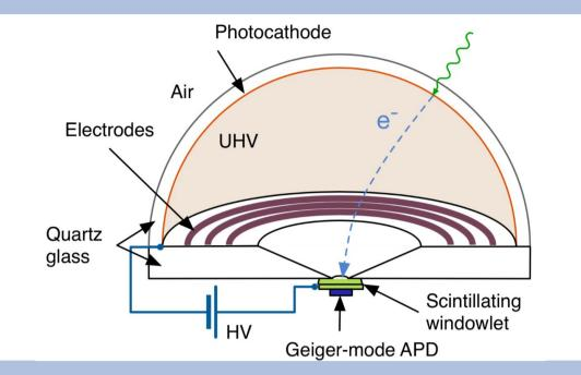
The scintillation light can then be from the read outside via an optically coupled silicon photomultiplier (SiPM).
