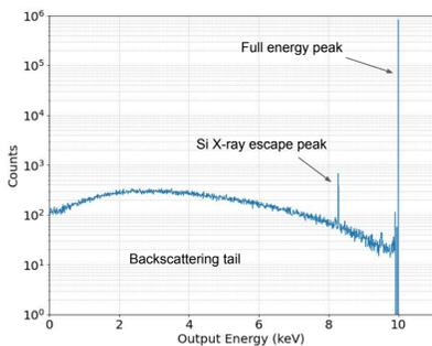
Raw spectrum: it includes backscattering electrons and escape X-rays
