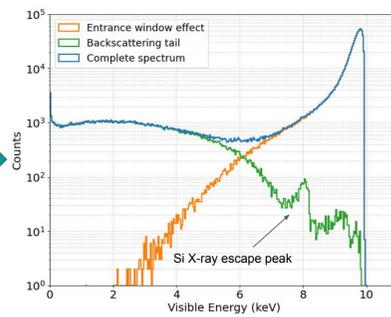
Apply weights to the energy deposited in the layers and sum up to obtain the total visible energy
