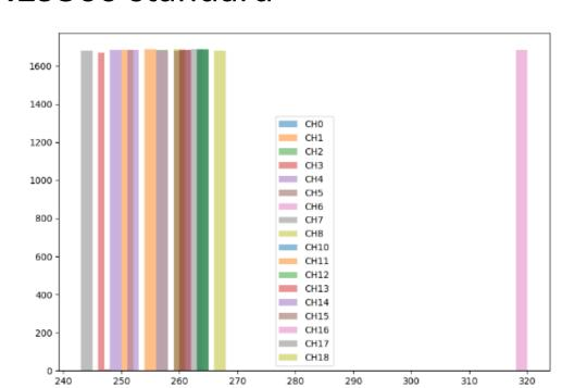
Pedestal of many FE acquired, the electronic noise is 1 LSB. Pedestal taken triggering with no signal on the input
