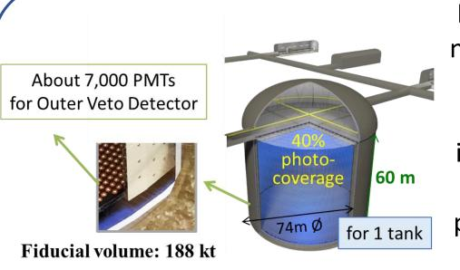
Hyper-Kamiokande is a next generation underground water Cherenkov detector designed to study neutrinos from astronomical sources, reactors and accelerators, nucleon decay, and with a focus on the determination of leptonic CP violation.
