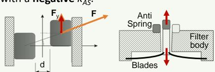
The total elastic force  $F = -(k_{blades} + k_{AS}) \cdot y$  is set to give a vertical frequency  $f_v = 0.3$  Hz.
