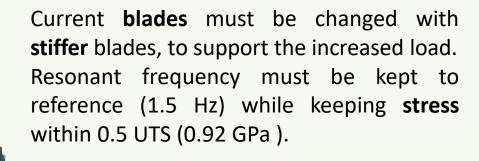
**Magnetic AntiSprings** must be re-tuned or re-designed to increase the antielastic constant  $k_{AS}$ .
