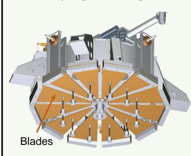
The springs are coupled with **magnetic** AntiSprings, exerting an force  $F = -k_{AS} \cdot y$  with a **negative**  $k_{AS}$ .
