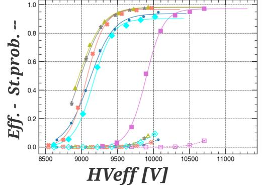
Novec 4710 and Amolea 1224yd tested with muon beam and gamma rate (~ 500 Hz/cm2)
