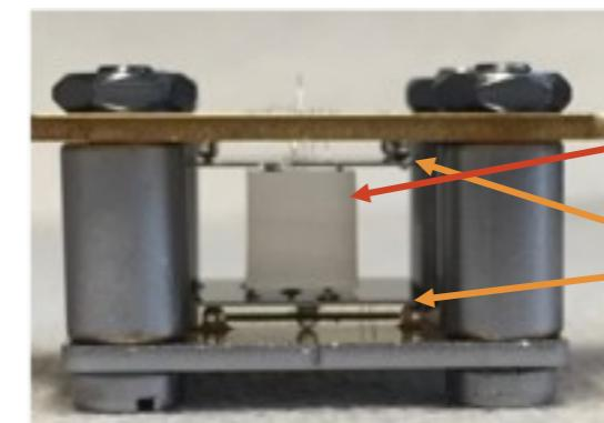
Target detector with ultra-low energy threshold of 20 eV<sub>nr</sub>
