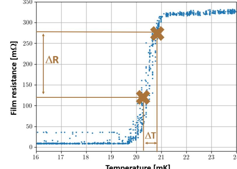
Temperature sensors on the detector's surface are based on superconducting thin tungsten films and are operated at a temperature in between of the normal to superconducting phase transition = Tungsten Transition Edge Sensors (W-TES)
