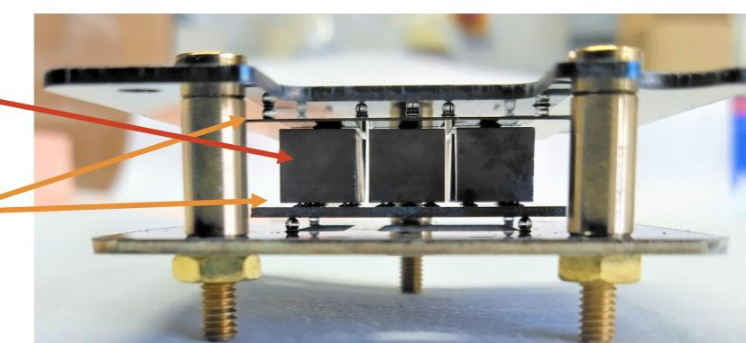
Mechanical set-up verified at room & cryogenic temperatures
