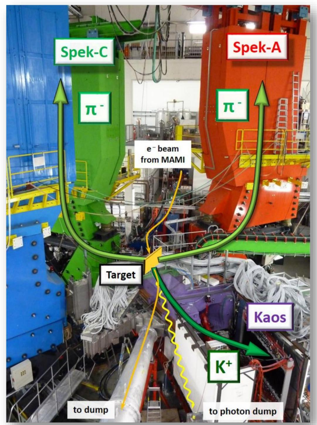
High-resolution decay-pion spectroscopy pioneered at Mainz Microtron (MAMI)
